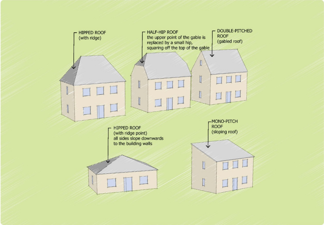
Figure 2: Technical terms for roof designs
