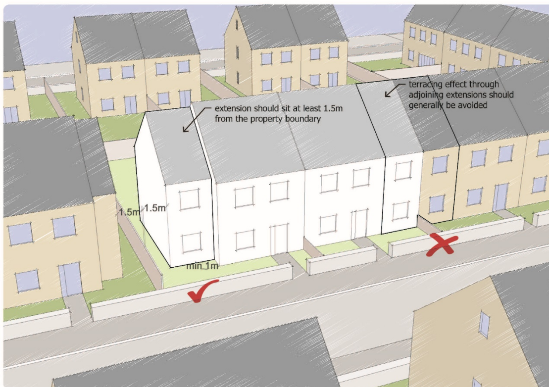
Figure 9: Side extensions and terracing effect
